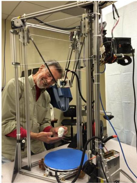
Rick displays a miniature “Yorick,” printed from polylactic acid (PLA) using the new custom-designed, custom-built 3D printer in the foreground.
