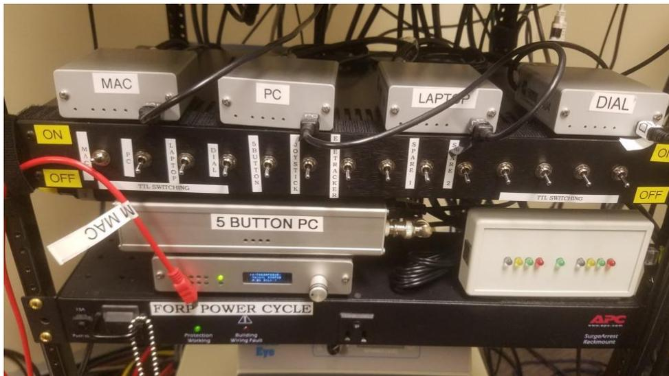
The new peripherals rack, with fORPs along the top of the toggle switch box controlling TTL reception.
