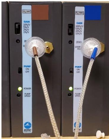
Figure 2 – CO2 and O2 BIOPAC Module w/Pumps
